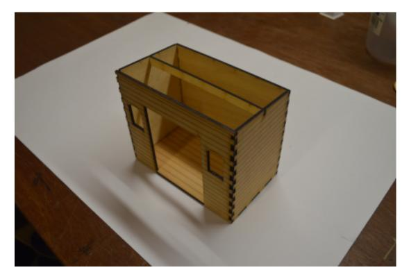
Assemble and glure together the front, sides and back to the floor ensuring that the engraved lines are facing outwards and that the engraved lines on the floor are facing up.
