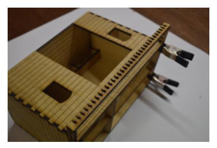
Glue the front detailing piece between the side pieces.
