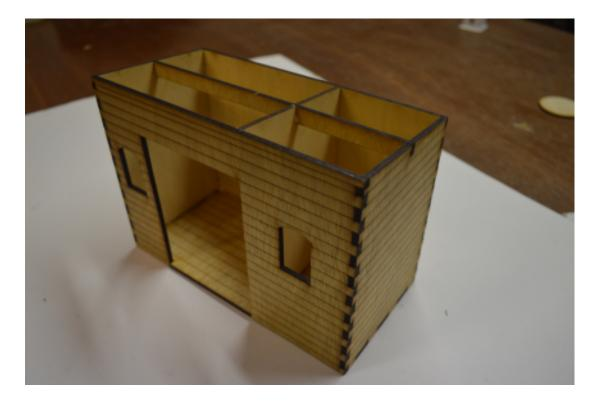
Assemble and glure together the front, sides and back to the floor ensuring that the engraved lines are facing outwards, the engraved lines on the floor are facing up and the engraved lines on the internal partition are facing inwards.
