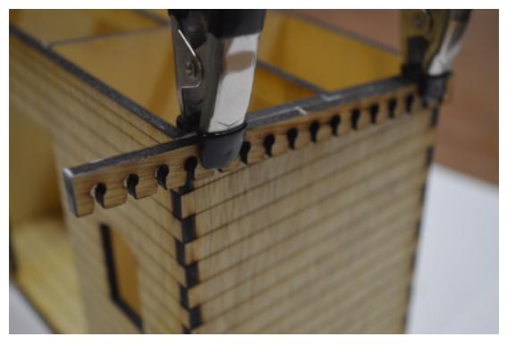
Glue and clamp the side pieces into place ensuring that the flat edge is lined up correctly with the back and the top of the side.
