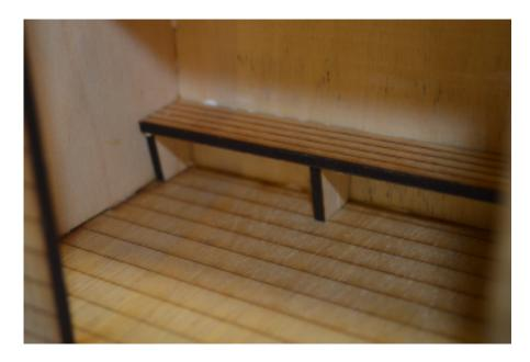
Glue the seat to the top of the seat supports and to the back ensuring that the engraved lines are facing up.
