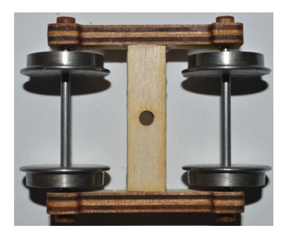
With the frames as shown in the picture below, glue the upper frame spacer on to the tabbed frame spacer ensuring that the holes line up.
