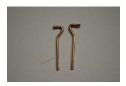
Cut 2 lengths of the supplied rod and form a hook at one end, ensuring that the rod is long enough to fit through all 3 buffers in the multi height coupling
