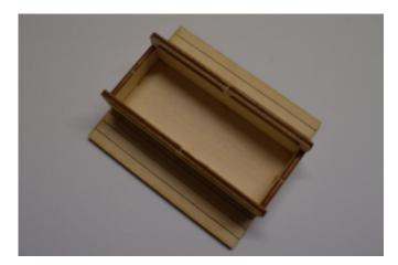
Assemble as shown ensuring that the engraved lines on the seat backs are facing outwards.
