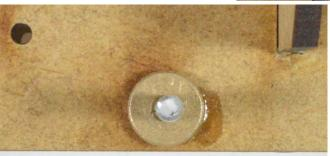
Locate the 2 axles and 4 wheel bearings and fit them as shown ensuring that the flange on the bearing is to the outside of the frames. Make sure that the axles are free to rotate in the bearings before gluing the bearings to the frames.
