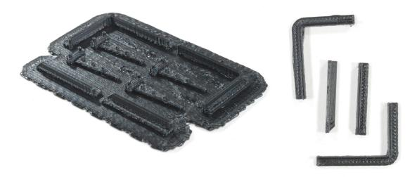
Locate the sprue with the 3D printed detailing parts and gently prize off the 4 frame detailing pieces. These can be removed by carefully sliding the blade of a modeling knive between them and the sprue.
