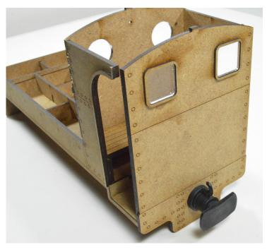
Fit the cab back to the rear inner buffer beam using the rear buffer to help line things up. With the model on a flat surface it will be resting on the front buffer beam and the cab rear piece with the frames raised slightly, this will help to line up the cab back verticaly. the 2 detailing pieces on the other side of the cab back should be just at the level of the cab floor, if not then trim them back with a sharp modeling knife.
