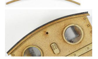
The final piece to fit is the cab front trim which should be fitted as shown in the photo to the left, after fitting it may need trimming off with a sharp modeling knife.
