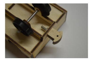
Finally fit the buffers and make up the coupling hooks using the supplied rod.
