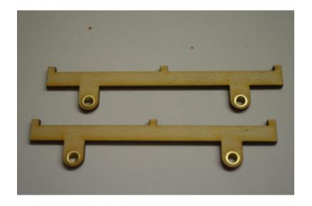
Press the bearings into the holes in the sole bars.
