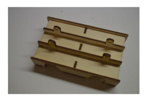
Fit the solebars into the locating holes on the underside of the floor ensuring that the flange of the bearings are facing outwards.
