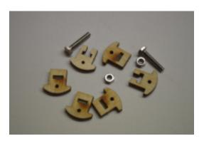
Locate the parts which make up the buffer. and glue all three sections together with the screw in the middle and the grooves on the outside pieces facing inwards to locate the screw head. Ensure that the small hole in all three parts line up so that the rod for the coupling can be passed through. Finally clamp all three sections untill the glue has set.
