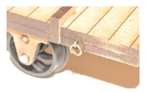
Finally bend 2 hooks from the supplied piece of steel rod and glue them into the holes on the wagon bed.
