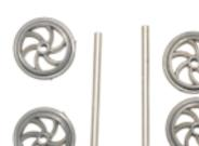
Assemble the wheels onto the axels with a flange to flange spacing of 28mm, ensuring that the flanges are inwards.
