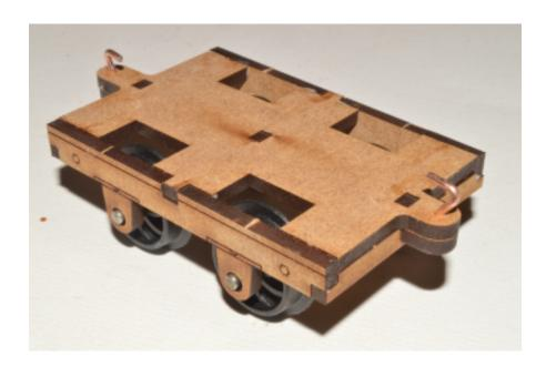
Glue the body onto the chassis using an all purpose adhesive such as UHU ensure that the body is flush with the back end of the chassis (the shorter buffer end) and overhangs at the front of the chassis (the longer buffer end)
