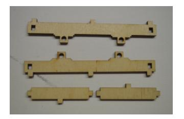
Locate the 4 parts that make up the inner chassis, these are 2 inner side pieces and 2 inner end pieces.
