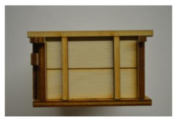
Fit both the end frames, ensuring that the engraved markings at the top of the verticals are facing outwards.
