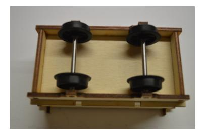
The inner chassis and wheels can now be fitted into the holes in the underside of the floor.
