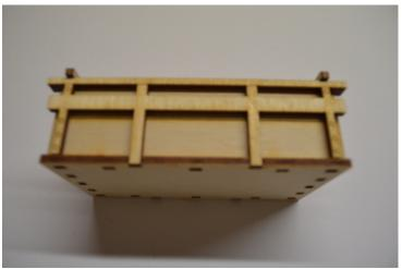
Fit both side frames by locating the middle longer frames into the cutouts in the floor ensuring that the engraved markings are facing outwards.
