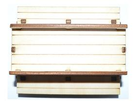
Glue the top box assembly onto the base unit assembly. If extra weight needs to be added then this should be done at this stage as the top box is capable of containing a substantial piece of lead.
