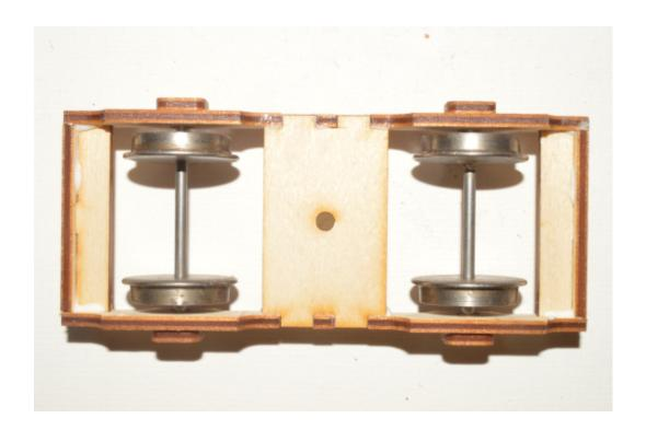
Glue the short and long centre frame spacers either side of the tabbed centre frame spacer ensuring that the holes in the centre line up.
