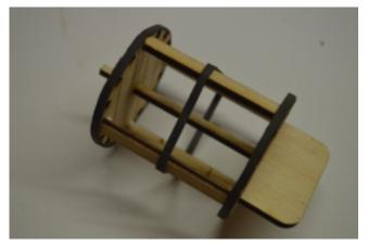
Assemble the rest of the slats onto the inner end pieces ensuring that the assembly is properly aligned and secure with an elastic band untill the glue dries.
