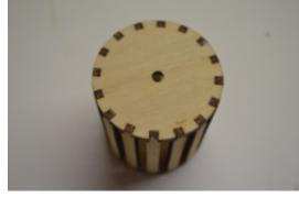
Once the glue has dried the assembly jig can be removed.
