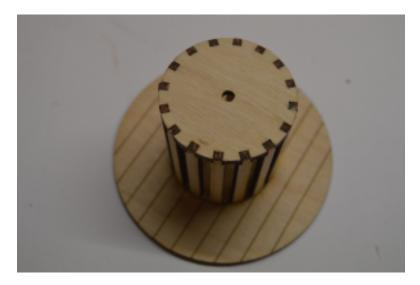
Glue the centre drum into the hole in the outer end piece ensuring that the 2 pieces are properly aligned and that the engraved lines are facing upwards and line up with the engraved lines on the end of the centre drum.
