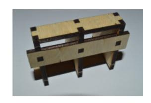
Glue and clamp the outer buffer beam to the inner buffer beam and the upper top piece to the lower top piece, ensuring the parts are correctly aligned.
