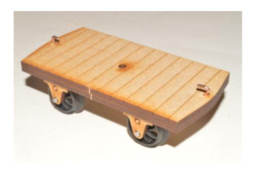
Locate the 6 pieces that make up the bolster, the M4 bolt head is sandwiched between the upper plain piece and the lower piece with the 4mm hole in it, the bolt head fits into the hex hole in the middle piece with the 2 side pieces locating the whole assembly together.
