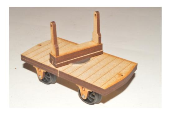
Assemble the bolster onto the chassis using a washer either side of the chassis bed and secured with the M4 nylock nut.
